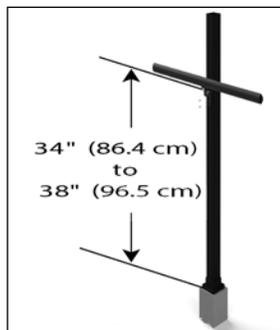
6. The maximum recommended span between supports is 6' (1.83 m) on center. Thus, placement of posts is critical when installation of railing is being considered.
